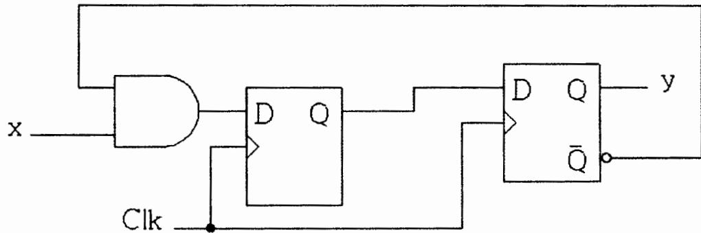
a) Determine the output ( $y$ ) waveform
